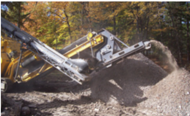
The RM80 compact recycler excels in small to medium scale recycling operations. Here, the RM80 and an excavator make their way through waste building material.
